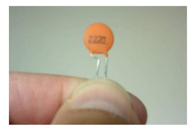
If the lead spacing of a capacitor are a little too wide for the hole pattern in the circuit board, they can be neatly bent with needle nose pliers to make a narrower spacing. Take care to not stress the lead where it enters the disc. I used the very tip of a very narrow pair of needle nose pliers to hold on to the lead where it exits the disc and a second pair of pliers to make the two bends.
